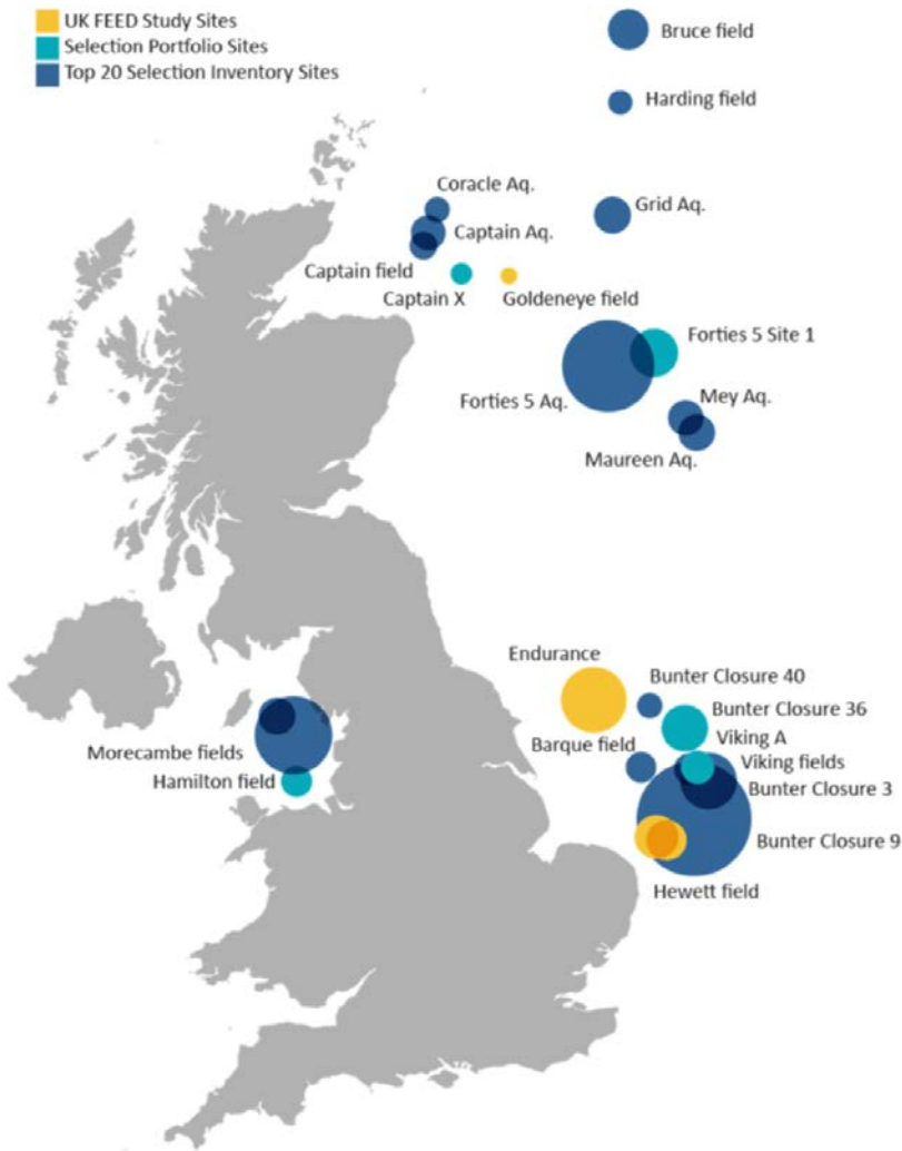
Figure 2-3 The UK inventory of 20 prospects and 8 matured sites: three early CCS competition FEED sites, and five later ETI strategic appraisal sites from 2016. Note the Mey prospect, Central North Sea, promoted as the ninth site in 2018.
