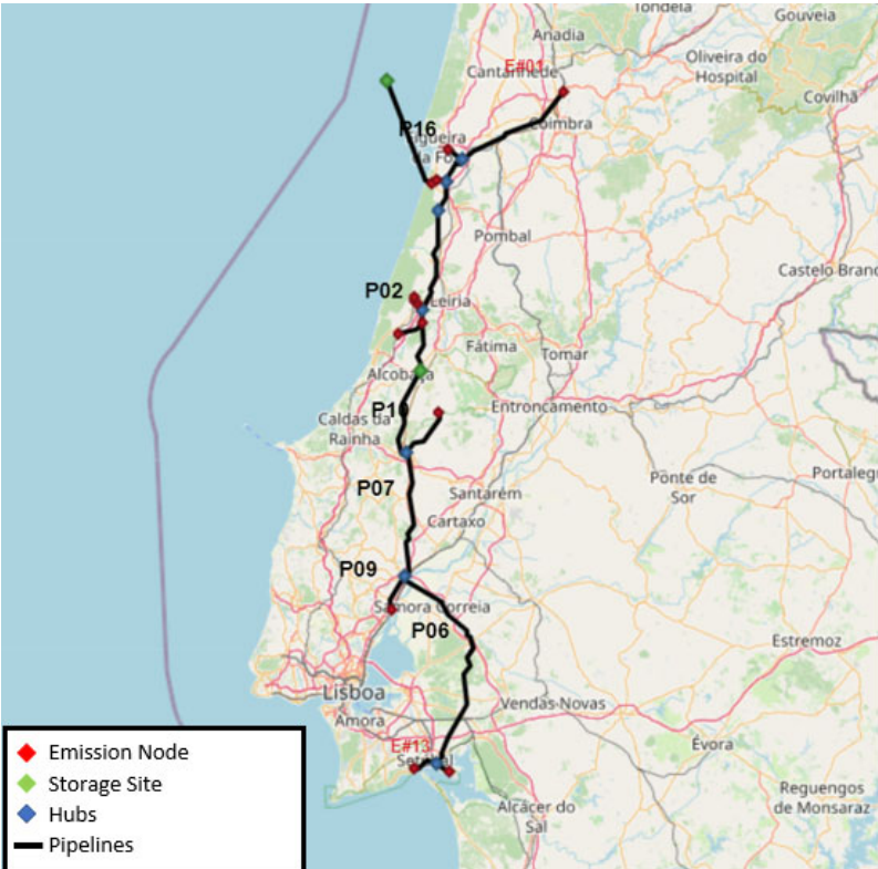
Figure 3.1-1: The geography of the emission clusters and the candidate pipelines and storage sites
