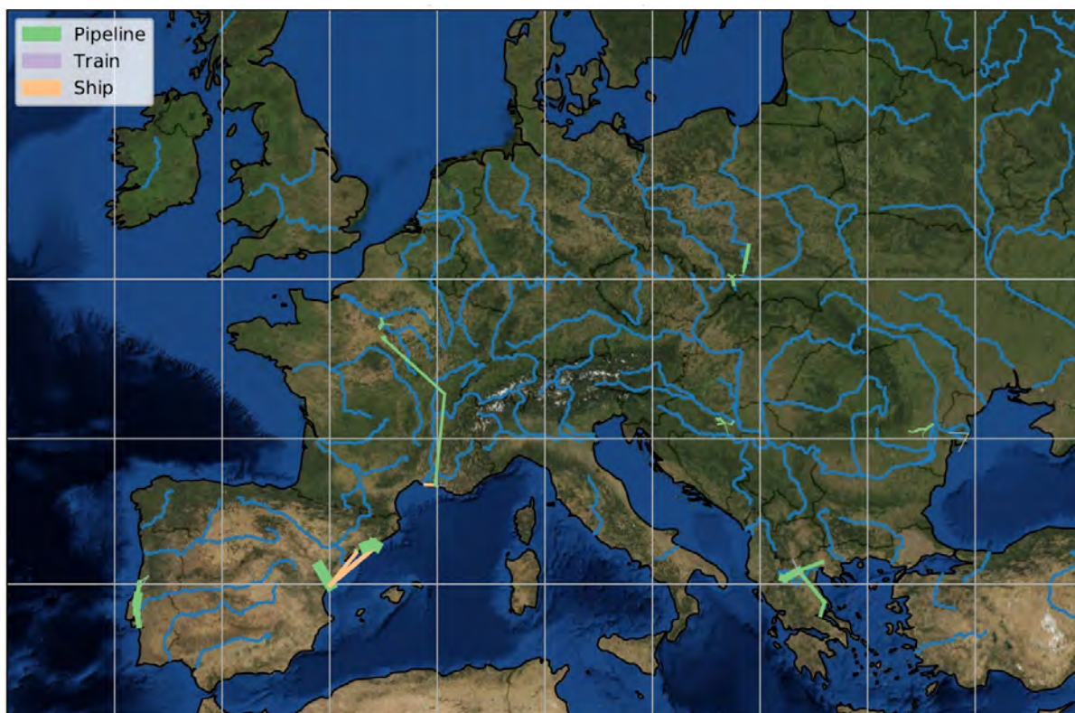
Figure 3: Regional transport network of the eight regional scenarios; Thickness of the line is proportional to the amount of transported CO 2
